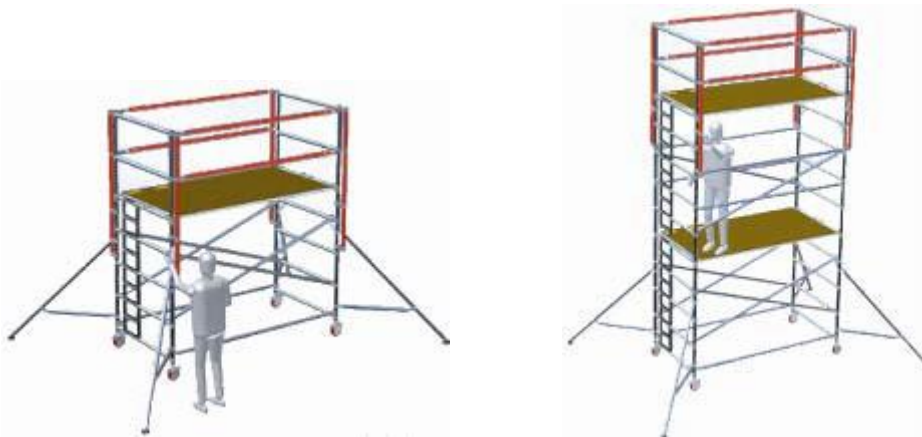
Figure 24: Advanced Guard-Rail Method for Erection of Mobile Towers
